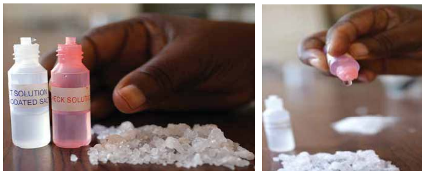
Figure 11: Testing salt for iodine using the rapid test kit
