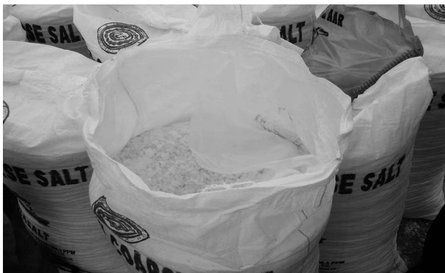
Figure 3: Inner lining for bulk salt packaging to prevent iodine losses
