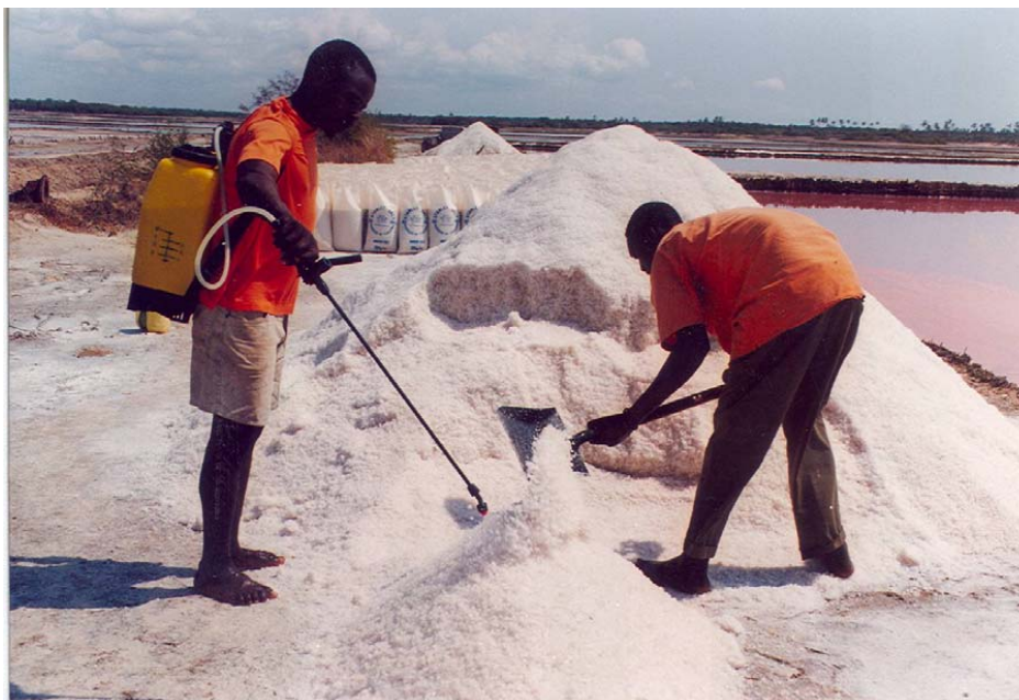
Figure 13: Salt iodation using knapsack sprayers with manual mixing
